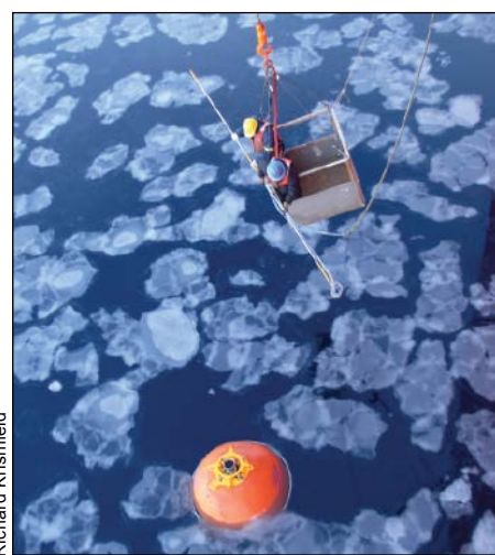
Recovery of a mooring top float with upward pointed ice thickness sonar in September 2010 amid pancake ice in the Beaufort Sea of the Arctic Ocean.
