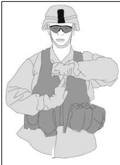
Figure 3-17. Load has not been released
