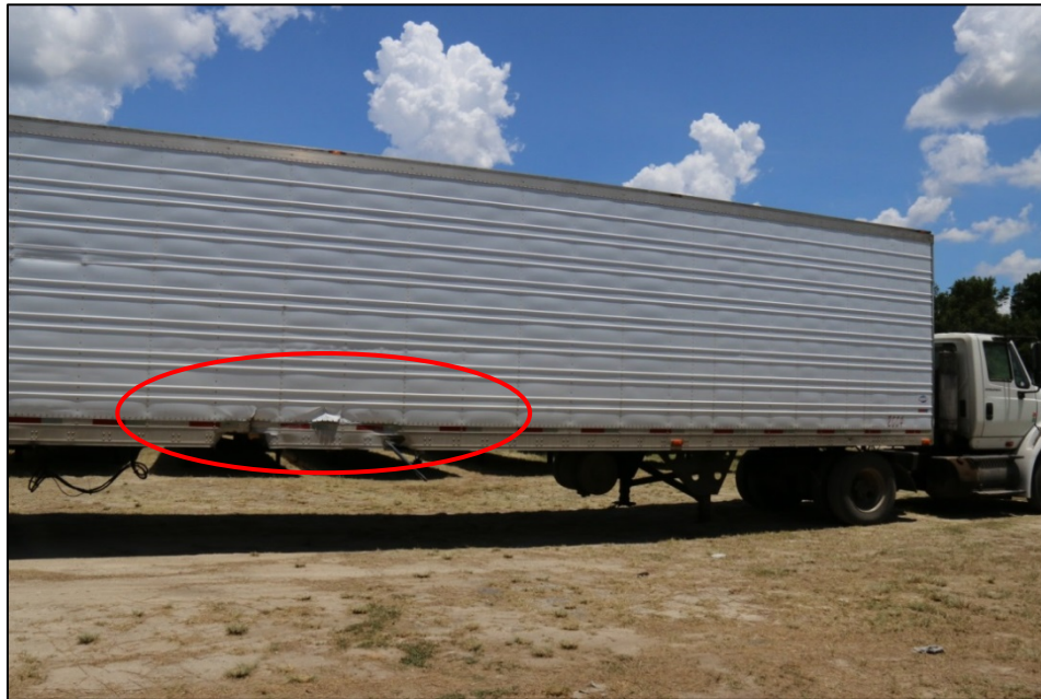
Figure 2. Right side of semitrailer. Area in red oval highlights collision damage from passenger car.
