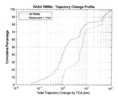
Note that some 35% of the maneuvers executed alter the trajectory more than 5km by TCA. If we plot just the large maneuvers, which we considered might be relocated DMUs, we still see several with relatively small trajectory alterations (about one-third are less than the 5km figure suggested by Amazon). Taken in an ensemble sense, these data indicate that the Amazon-recommended figure is not adequate as submitted. Instead, our recommendations are the following:
