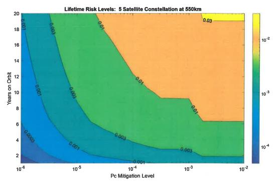
Here the ODPO requirement contour is now between the blue and aqua colors (labeled 0.001), and one sees that it cannot be met at all at a mitigation level of 1E-04 and for constellation lifetimes of only about
