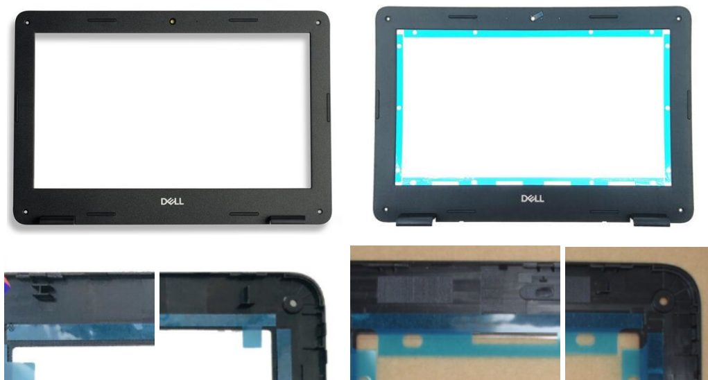
Figure 7. Can you spot the difference? From left to right, on top the front and on the bottom the back of the Dell 11 3100 Non-touch Chromebook Bezel and Dell 11 3110 Non-Touch Chromebook Bezel. These parts are not compatible across models, the only external changes between them being the addition of small notches on the bottom of the newer model. On the bottom row from left to right, on the back of the bezels we can see that 3110 has missing or less pronounced clips which renders them incompatible. Image credit: edu-parts.com
