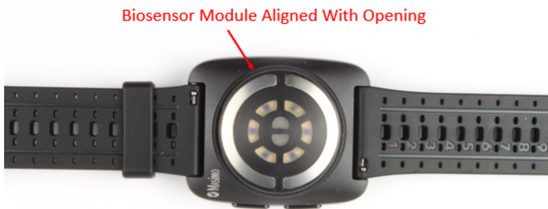
(FCC MASIW1 Masimo W1 Internal Photos (annotations added)).
